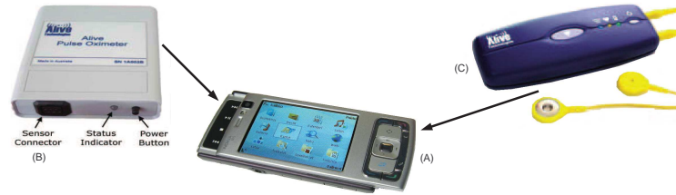
Fig. 1. The Nokia N95 cellphone fusion center (A), and the Alive Technologies oximeter sensor (B) and ECG sensor (C).
