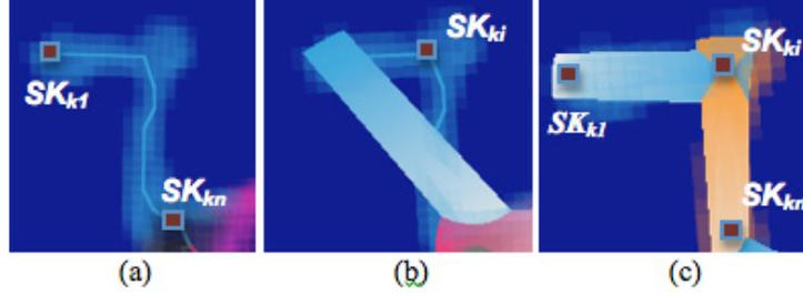
**Fig. 4.** The coarse-to-fine approximation process: (a) the decomposed part  $P_k$  of the skeleton within the range of  $[SK_{k_1}, SK_{k_n}]$ , (b) the decomposed part  $P_k$  is approximated by a single d-cylinder and the slice with the max distortion error is found at  $SK_{k_i}$ , and (c) the old d-cylinder is divided at  $SK_{k_i}$  and replaced by two new d-cylinders.
