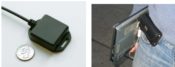
(a) MotionNode platform (b) During data collection, MotionNode is packed firmly into a mobile phone pouch and attached to the subject’s front right hip
