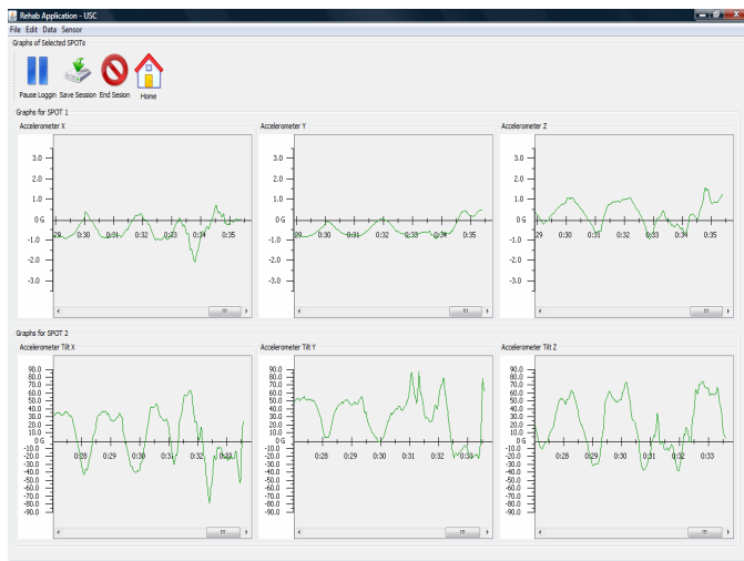
Fig. 8. A snapshot of the data captured from the two free-range nodes where the patient was slowly moving his left arm up and down
