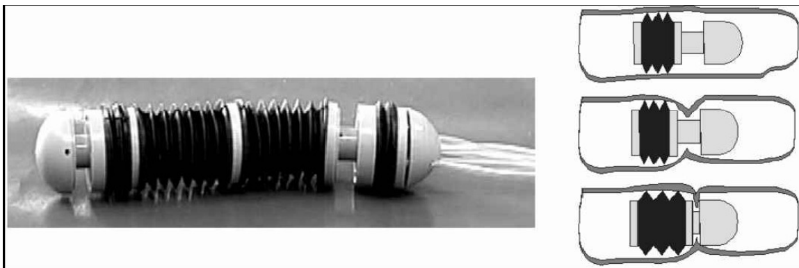
Figure above shows the gait sequence of the forward propulsion (Dario et al. 1999).
