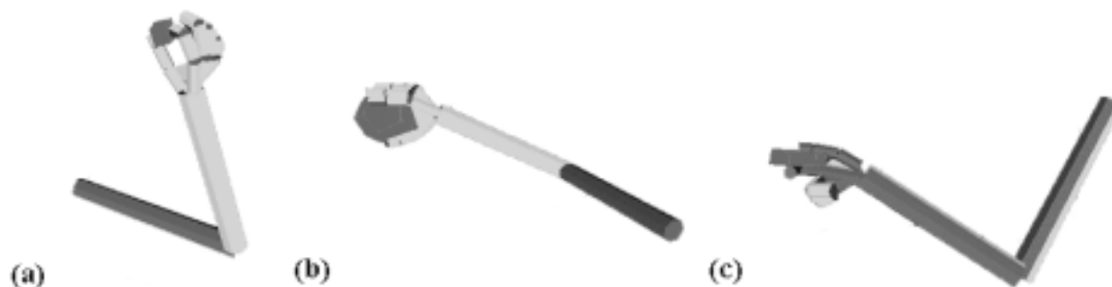
Figure 10. Grasps generated by the simulator. (a) A precision grasp. (b) A power grasp. (c) A side grasp.
