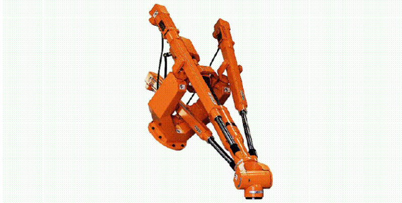
Figure 1.18: The ABB IRB940 Tricept parallel robot. Parallel robots generally have much higher structural rigidity than serial link robots. (Photo courtesy of ABB.)
